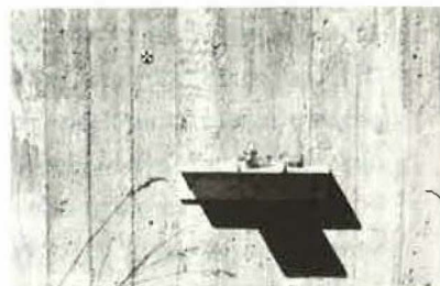
Figure 1. The reference point target on the test wall and the centered scale reference point.
