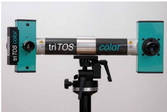
Figure 3. triTOS fringe projection system
