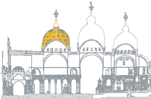
Figure 4. The 2D representation of Pentecoste wooden beams into the Basilica longitudinal section
