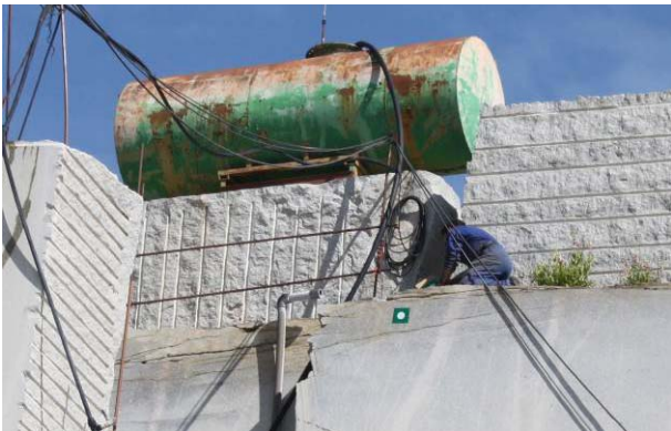
Figure 3. Artificial target located in the vertical wall of the quarry
