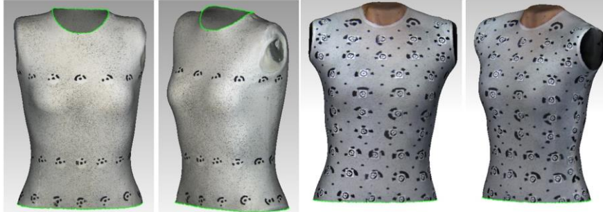
Fig. 1: Three-dimensional digital models obtained with the proposed body scanning system.
