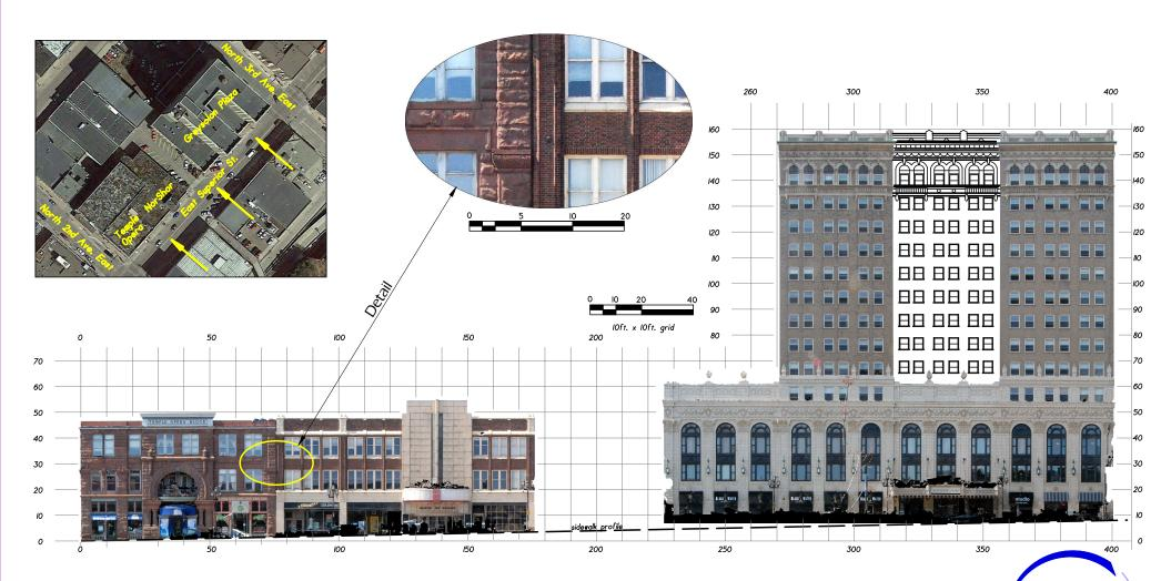
Orthophoto of structures to 65' above ground Rectified photos of structures above 65' CAD rendering of central portion of Greysolon Plaza
